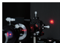
Diffraction rings produced when the focus spot is smaller than the pinhole diameter
