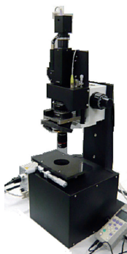
Coaxial observation system with phase difference measuring system
